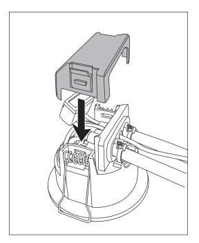
**7.** Insert the device with the mounting folded up into the installation opening.
